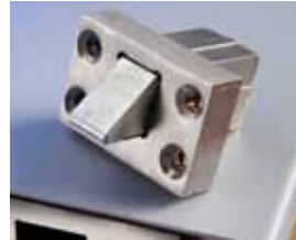
Top Latch 5/8" stainless steel housings, 3/4" projection with 1/8" door gap
